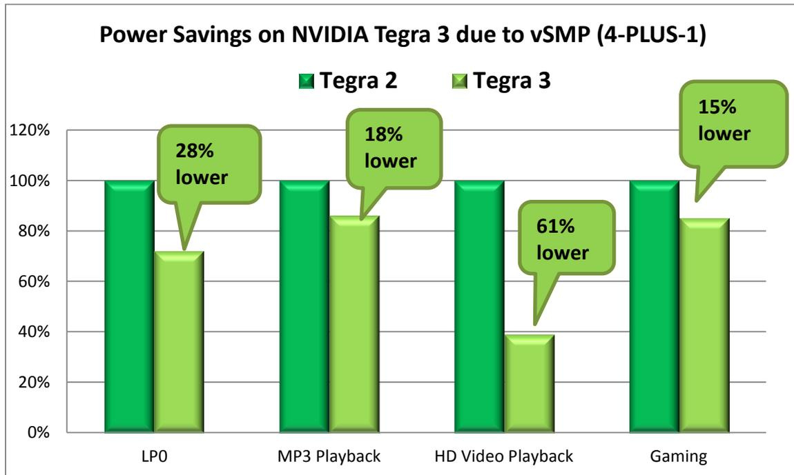
Figure 6 Power savings on NVIDIA Tegra 3 due to vSMP (4-PLUS-1)<sup>1</sup>
