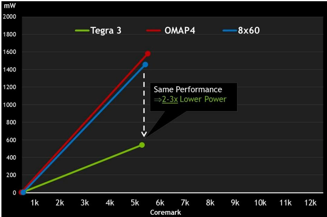
Figure 7 Tegra 3 power consumption when delivering the same performance as competing dual core processors<sup>7</sup>
