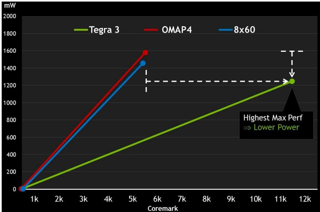
Figure 8 Tegra 3 power consumption delivering maximum quad core performance<sup>8</sup>
