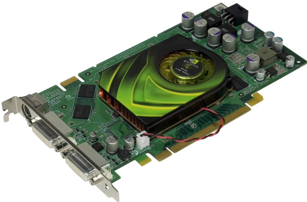
Figure 3: A modern Windows Vista Aero capable graphics add-in card
