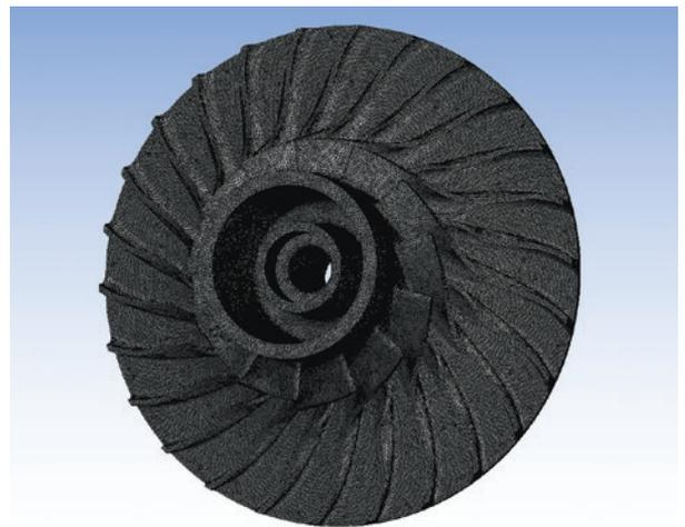
▲ Radial impeller cyclic symmetry model (visually expanded)
