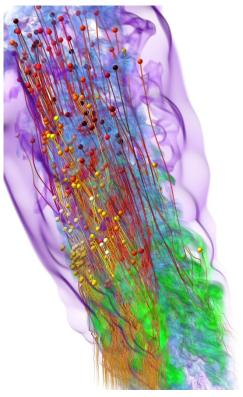
S3D combustion code: lifted ethylene-air jet flame computed from DNS and tracer particle trajectories. C.S. Yoo and J. Chen performed the DNS. H. Yu (Sandia); R. Grout of the NRELperformed volume rendering.
