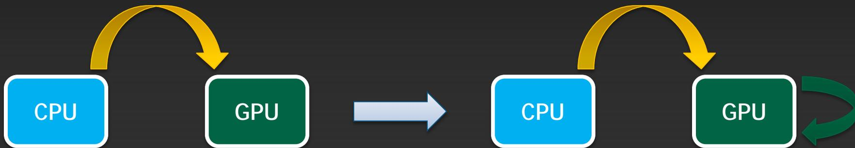
*Fermi: Only CPU can generate GPU work*
